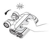
When replacing, always latch the brush cover into place to avoid leakage.
