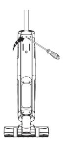
In the event that the handle needs to be disassembled, press the spring to release the handle with a tool (like a screwdriver) and lift the released handle from the appliance.
